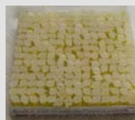
Storage of plasma samples in 0.2 mL PCR tubes (they need only a quarter of the usual volume and can be directly used in the pipetting machine)
