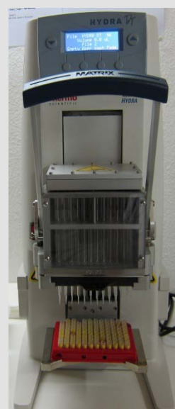
Pipetting machine with the 0.2 mL PCR tubes
